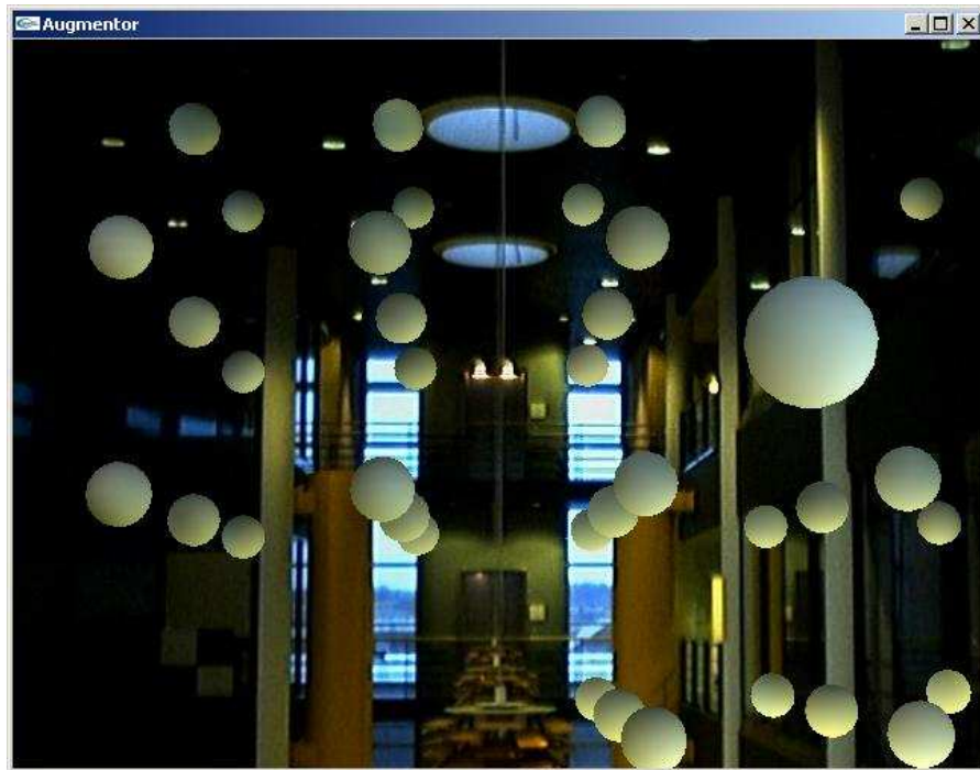
Figure 13.3: The samples created in the irradiance volume is displayed in the lobby scene.
