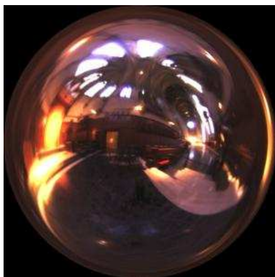
(a) An example of an angular map used by [Debevec, 1998] extracted from images of a light probe.
