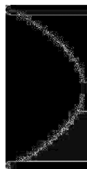
Figure F.7: The errors of the JPEG compression appears as white dots on the background, the whiter the dots, the greater the error.
